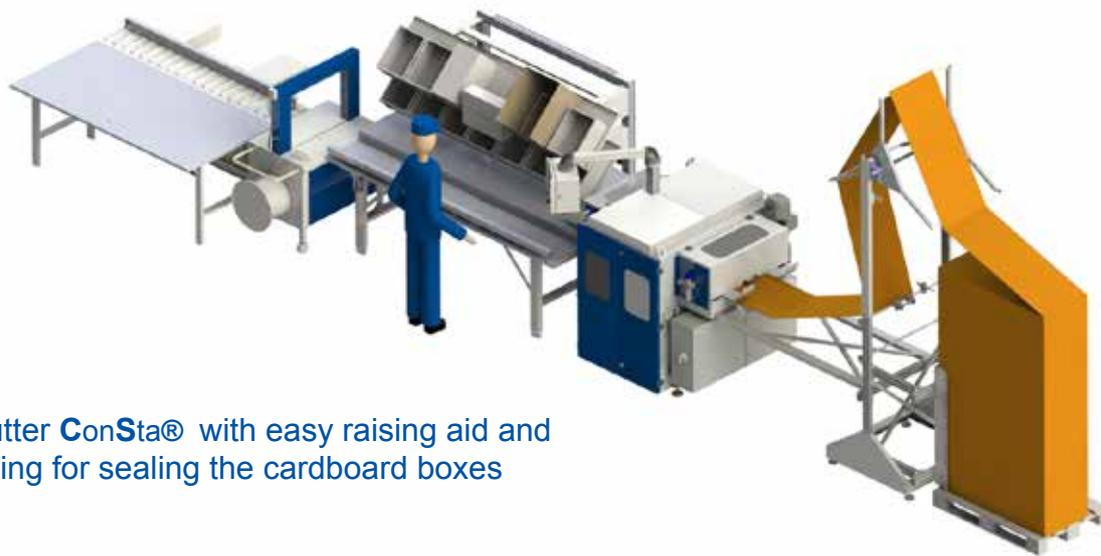
Die-cutter **ConSta®** with easy raising aid and strapping for sealing the cardboard boxes
